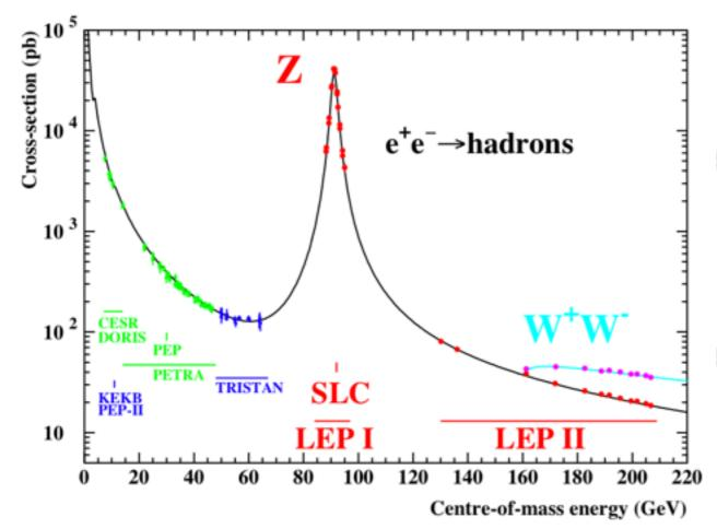
lineshape: cross section scans at circular lepton colliders (energy calibration through resonant spin depolarization)
