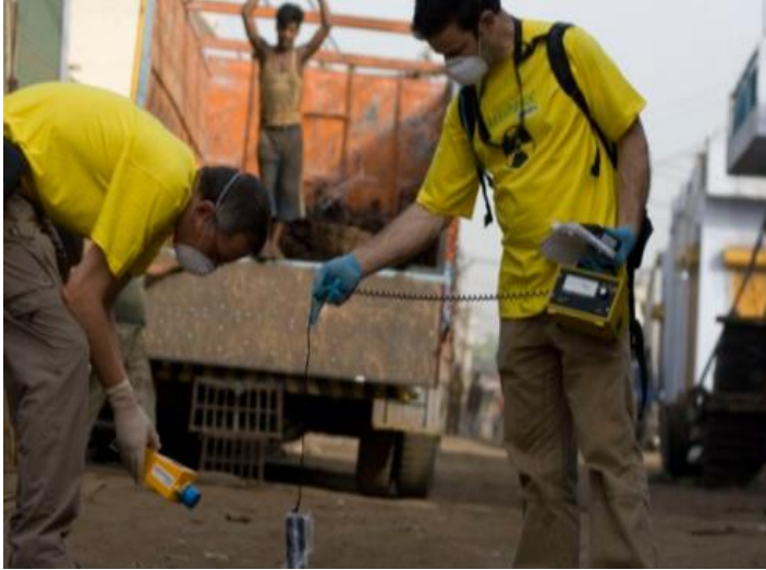
Recovery of Co-60 pencils from a scrapped teletherapy unit in India
