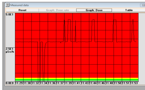
Dose Rate: 0.2 cGy/min @ 670kW RF Power Injection
