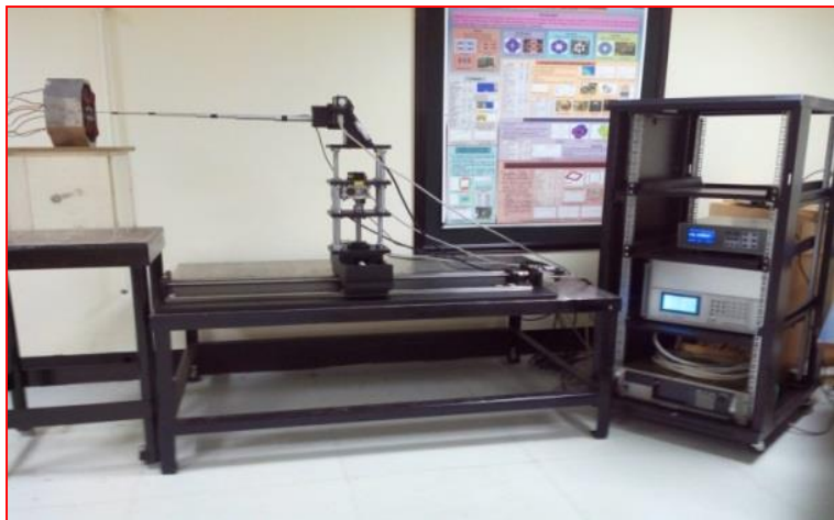
Hall Probe Magnetic Measurement System
