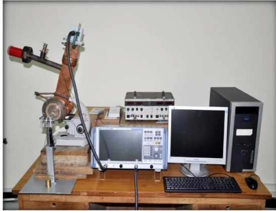
Indigenously developed Bead pull setup
