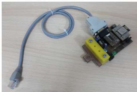
Power Supply Remote Controller
