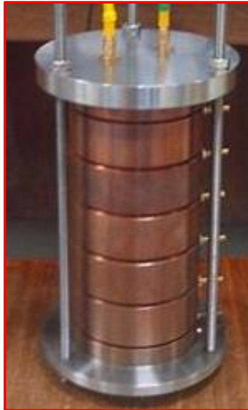
Traveling Wave Accel. Structure
