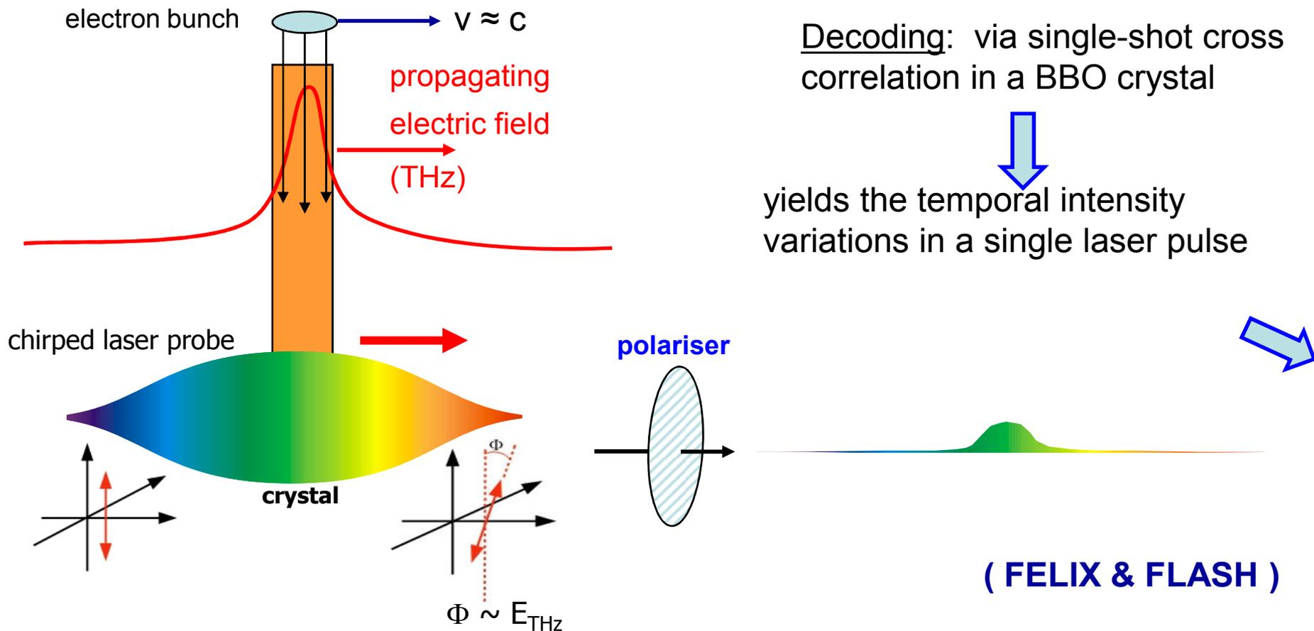
Detect polarisation rotation proportional to  $E$  or  $E^2$ , depending on set-up
