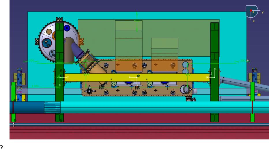
Interference with cable trails (longer beam)
