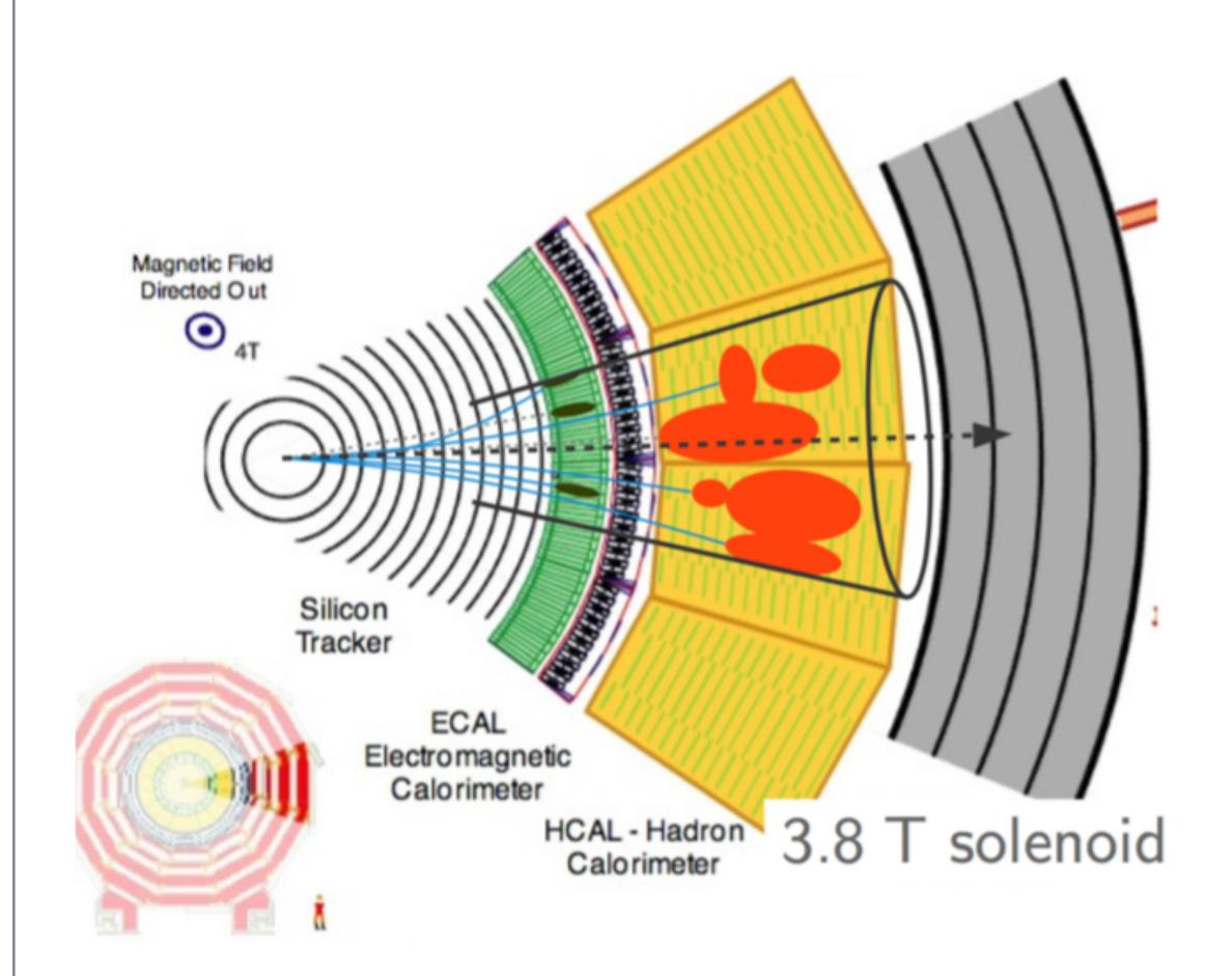
Jet reconstruction uses the information from the silicon tracker, ECAL and HCAL Each jet then needs to be calibrated
