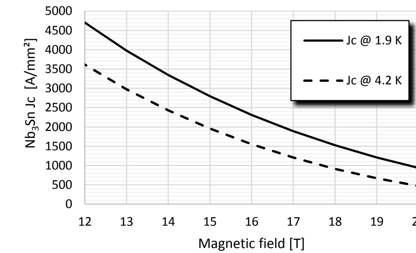
$$\begin{cases} J_c = \frac{C(t)}{B} b^{0.5} (1-b)^2 \\ B_{c2}(T) = B_{c20} (1-t^{1.52}) \\ C(t) = C_0 (1-t^{1.52})^\alpha (1-t^2)^\alpha \end{cases}$$
