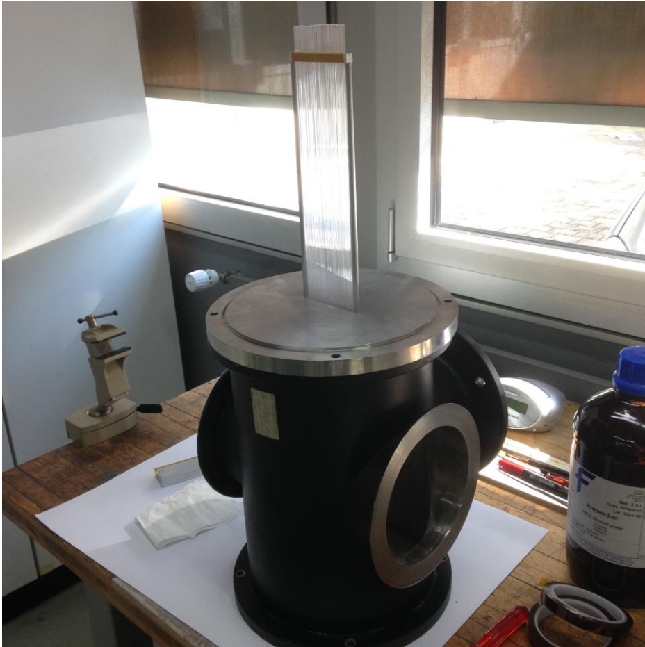
The array of fibres hanging upside-down for glue drying
