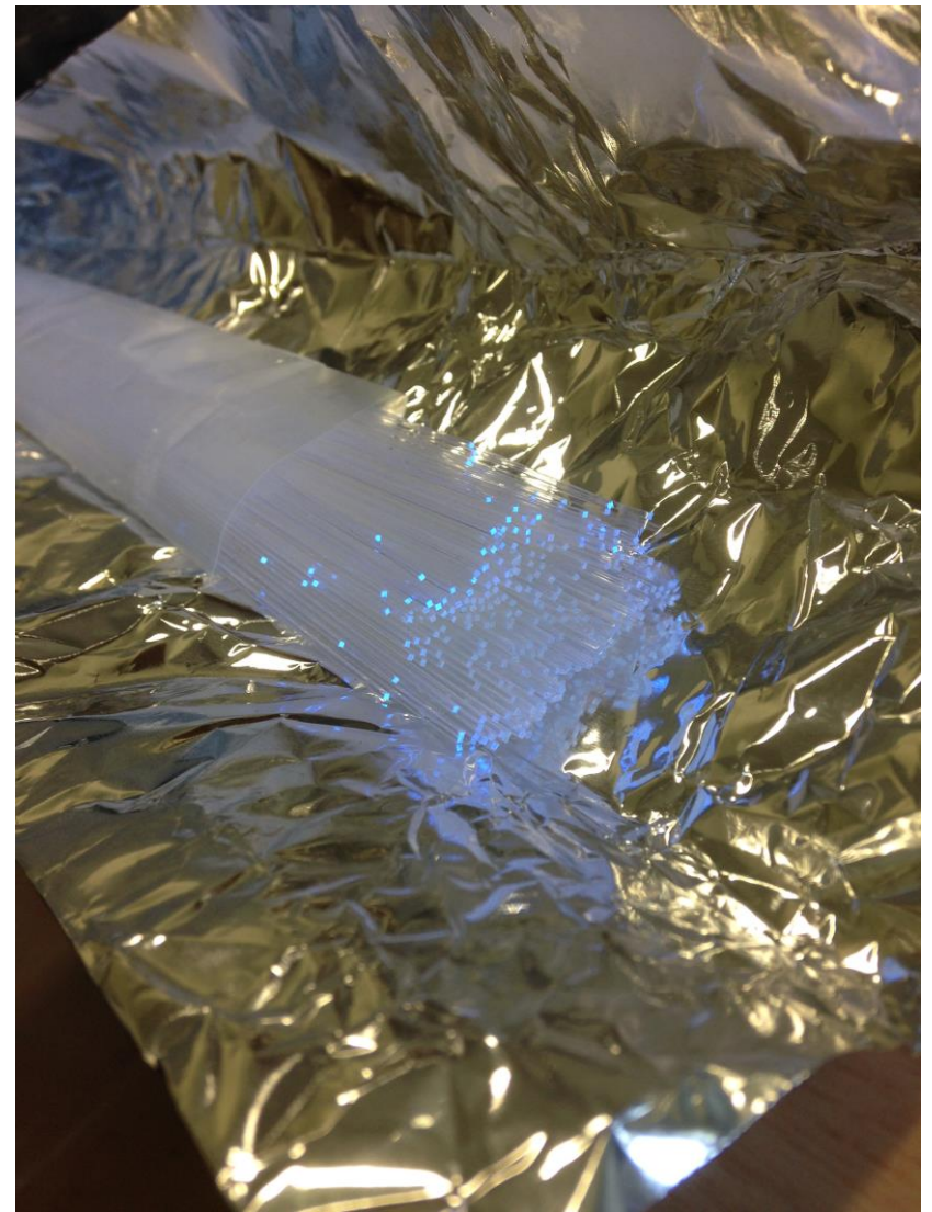
The fibres used: Saint-Gobain BCF12, 1mm square, multi-cladding
