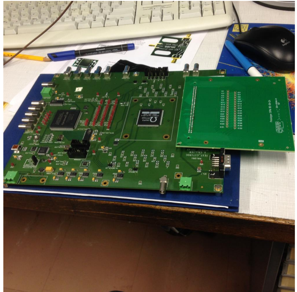
The MPPC board plugged onto the CITIROC board
