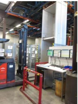
One Carrier (2 shelfs) at the loading station waiting for Pallets to be inserted
