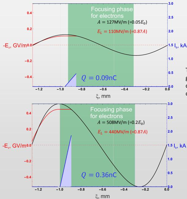
A – wakefield amplitude  $n_0 = 7 \cdot 10^{14} \text{ cm}^{-3}$  – plasma density  $E_0 = 2.54 \text{GV/m}$  – wavebreaking field  $E_L$  – loaded wakefield magnitude Q – beam charge
