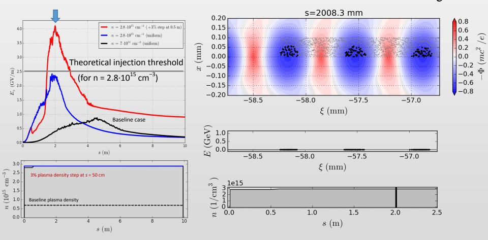
Just 3 mm is necessary to reach 10 MeV! (10 MeV / 3 mm = 3.3 GeV/m)
