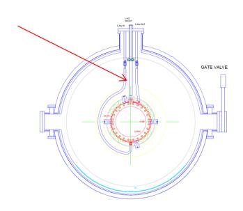
Heater installed on Hydrogen return pipe.
