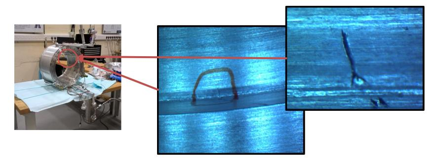
Surface defects – x-ray and dye penetration test showed no results
