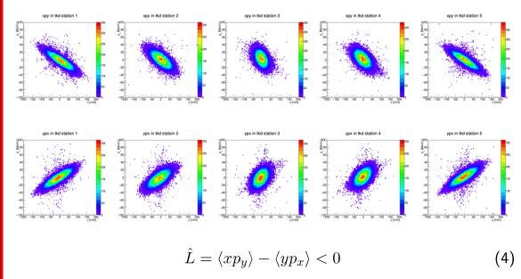
$\rightarrow$  Anticlockwise rotation, **normal** polarity
