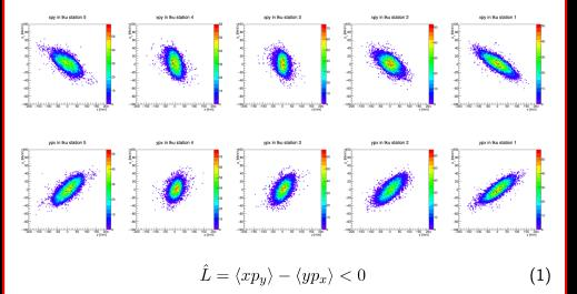
$\rightarrow$  Anticlockwise rotation, **normal** polarity
