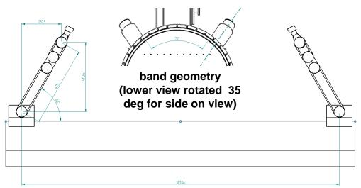
\*Actual movement where bands slip & total drop in height is dependant on stiffness of bands + gravity effects, however assuming further ~ 4 mm of movement [from 1 mm to 4.81 mm] the drop in height of the end of the bobbin could be as shown in the adjacent table [based purely on geometric rotation from 60 degrees of bands then reduced for 35 degree angle]
