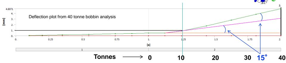
With this set-up @ 11 tonnes ~ 1 mm of axial bobbin movement occurs before the bands slip their pins\*. The bands on the bottom would lose control of the bobbin at this point but those on top would still be in contact, however as the bobbin moves axially further the top bands would rotate between their anchor point on the OVC and their anchor point on the bobbin potentially changing the height of the bobbin on the slack band end
