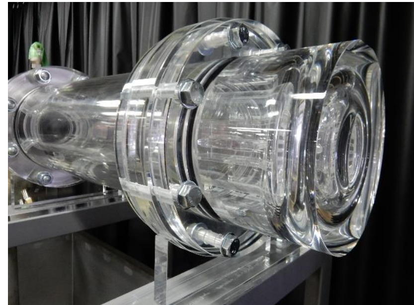
Test device for flow visualization by PIV method (Full-scale transparent acrylic model of target vessel
