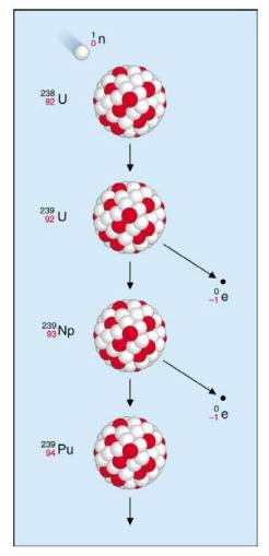
Neutron capture of U238, followed by beta-decay of U239 and continuation of this process leading to Pu239 (and beyond)
