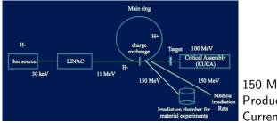
150 MeV proton FFAG ring Producing useful beams Current  $\sim 1nA$
