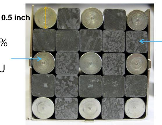
solid Pb coolant simulator and reflector
