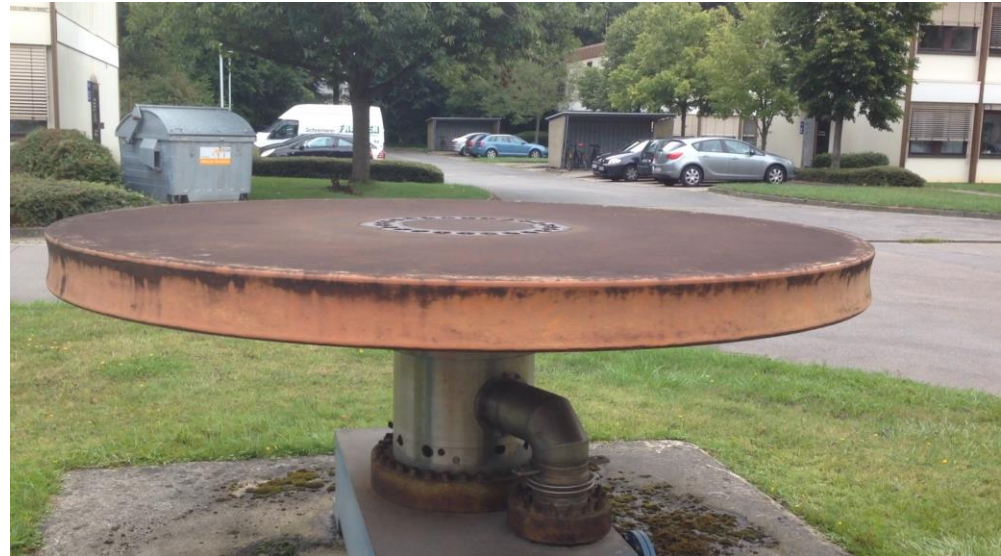
Prototype rotating target from the 1980s-era German SNQ project (Forschungszentrum Jülich)
