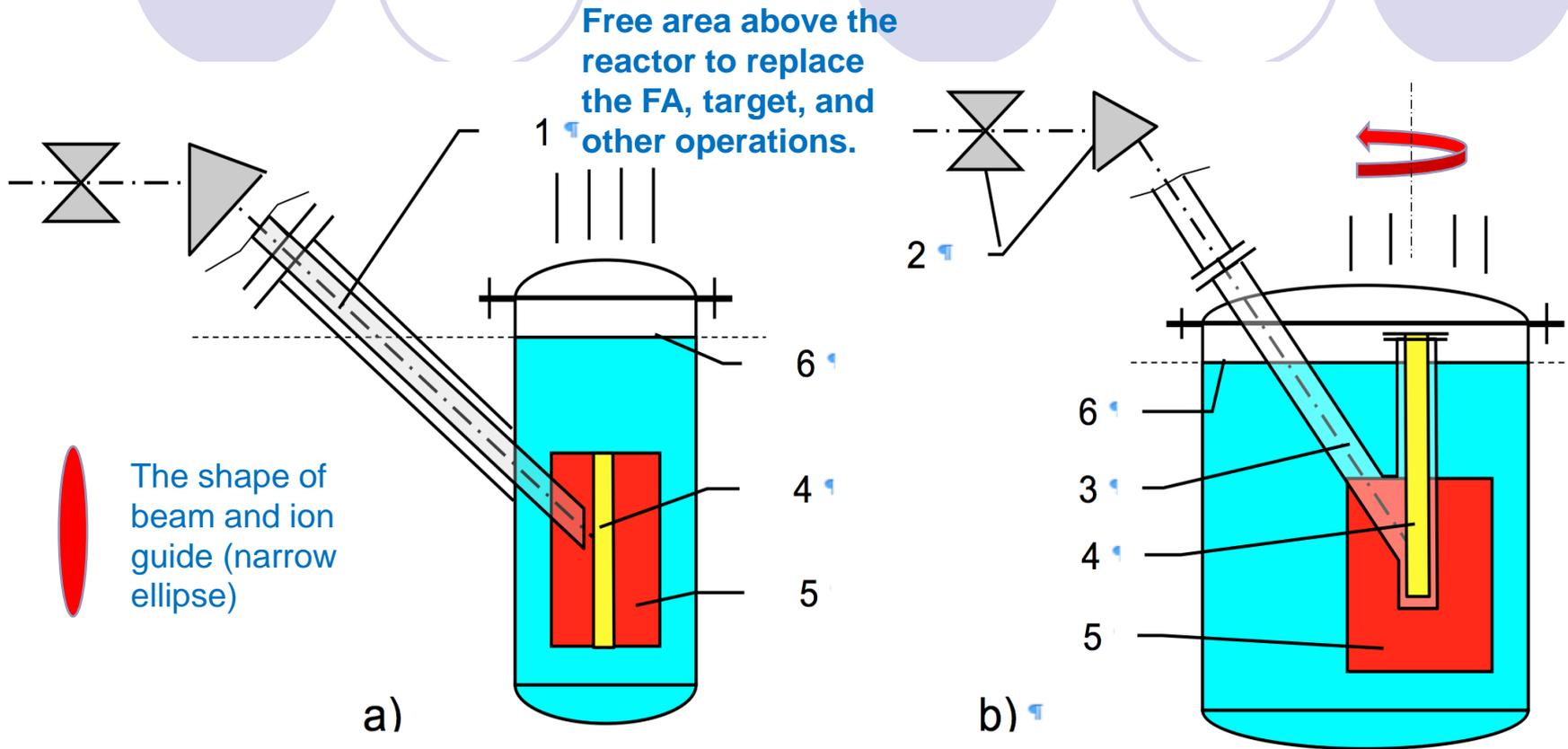
Schematic of the input of a proton beam diagonally (sideways from above): (a) with separate cooling window on the removable portion of the ion guide; (b) with placement of target module inside vacuum chamber that is connected with the proton guide.
