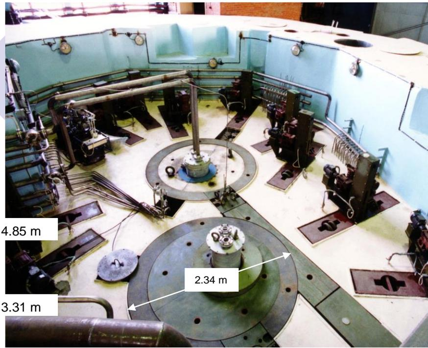
*The scheme of the second cell in the shield and its basic sizes*
