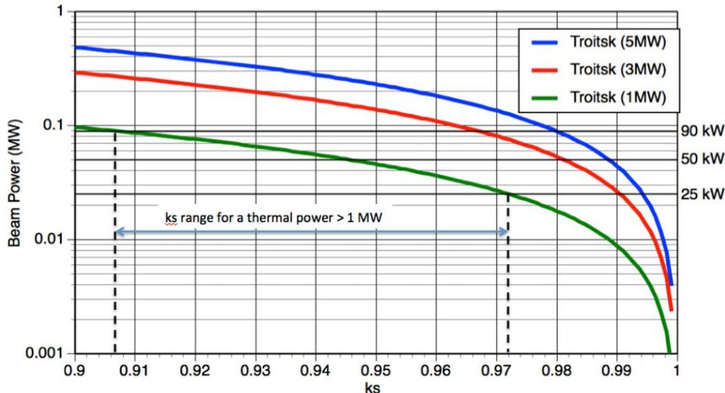
With the achievable accelerator parameters the 1 MW line (green) looks realistic.
