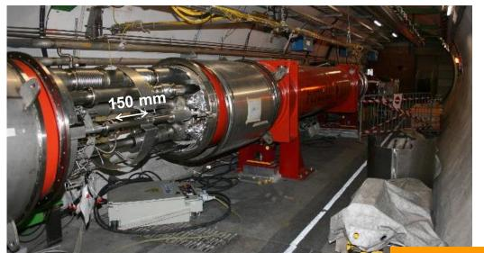
"modular sputtering source" pulled by cables all along a magnet
