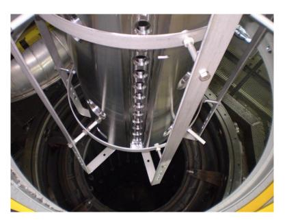
The **CERN's large furnace**: useful height and diameter: 6 m and 1 m, respectively. Maximum charge weight: 1000 Kg. Ultimate pressure: about 10<sup>-7</sup> mbar; pressure at the end of the 950°Cx2h treatments: 10<sup>-5</sup>mbar.
