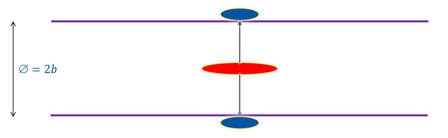
Image charges flow on the surface of the beampipe
