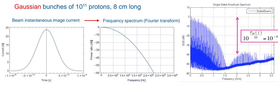
Power dissipation from wakes is  $P_{loss} = MI_b^2 \operatorname{Re}(Z_s^{eff})$
