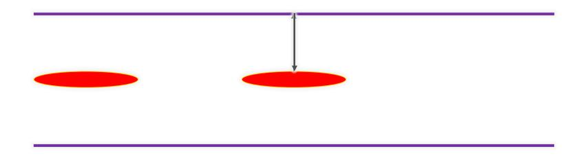
Wakefields have an effect on beam stability, in particular the transverse plane Risetime of resistive-wall instability depends on the transverse impedance
