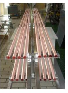
Mechanical removal of most of the Cu particles (Clothing and 100 bar water rinsing).
