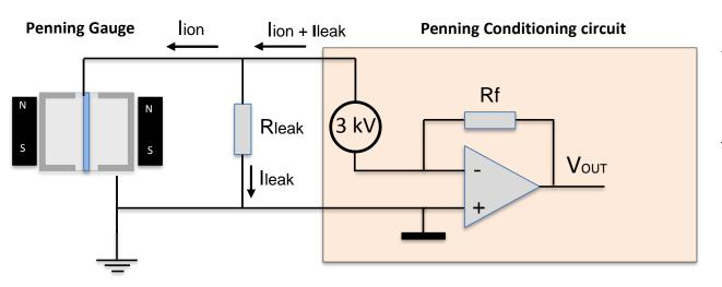
$$V_{OUT} = R_f \cdot (I_{ion} + I_{leak})$$
