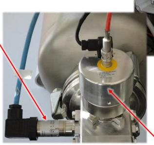
Penning electronics Pirani custom electronics 24VDC supply 0-10V output Used in **low** radiation areas
