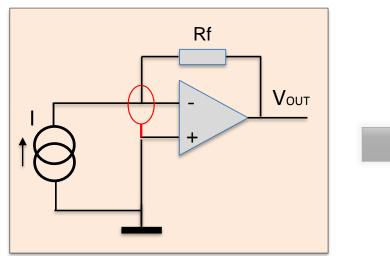
$$V_{OUT} = R_f I$$
