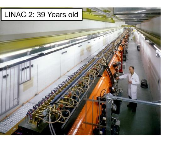
LINAC 2 started up in 1978 when it replaced LINAC 1. It was originally built to allow higher intensity beams for the accelerators that follow it in CERN's accelerator complex. LINAC 2 will be replaced by LINAC 4 in 2020.
