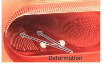
Beam induced, via impedance, thermal outgassing
