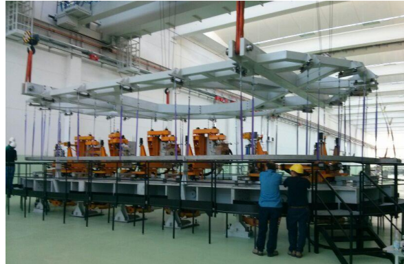
ITER TF coil insulating machine
