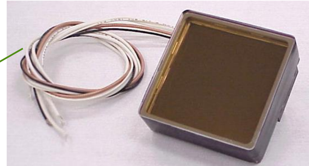
25 \mu\text{m} pore size; 5.3x5.3 cm 2 active area; 64 pixels (8x8), 6.5 mm pitch per pixel; rise time \sim 0.6 ns, pulse width \sim 1.8 ns.
