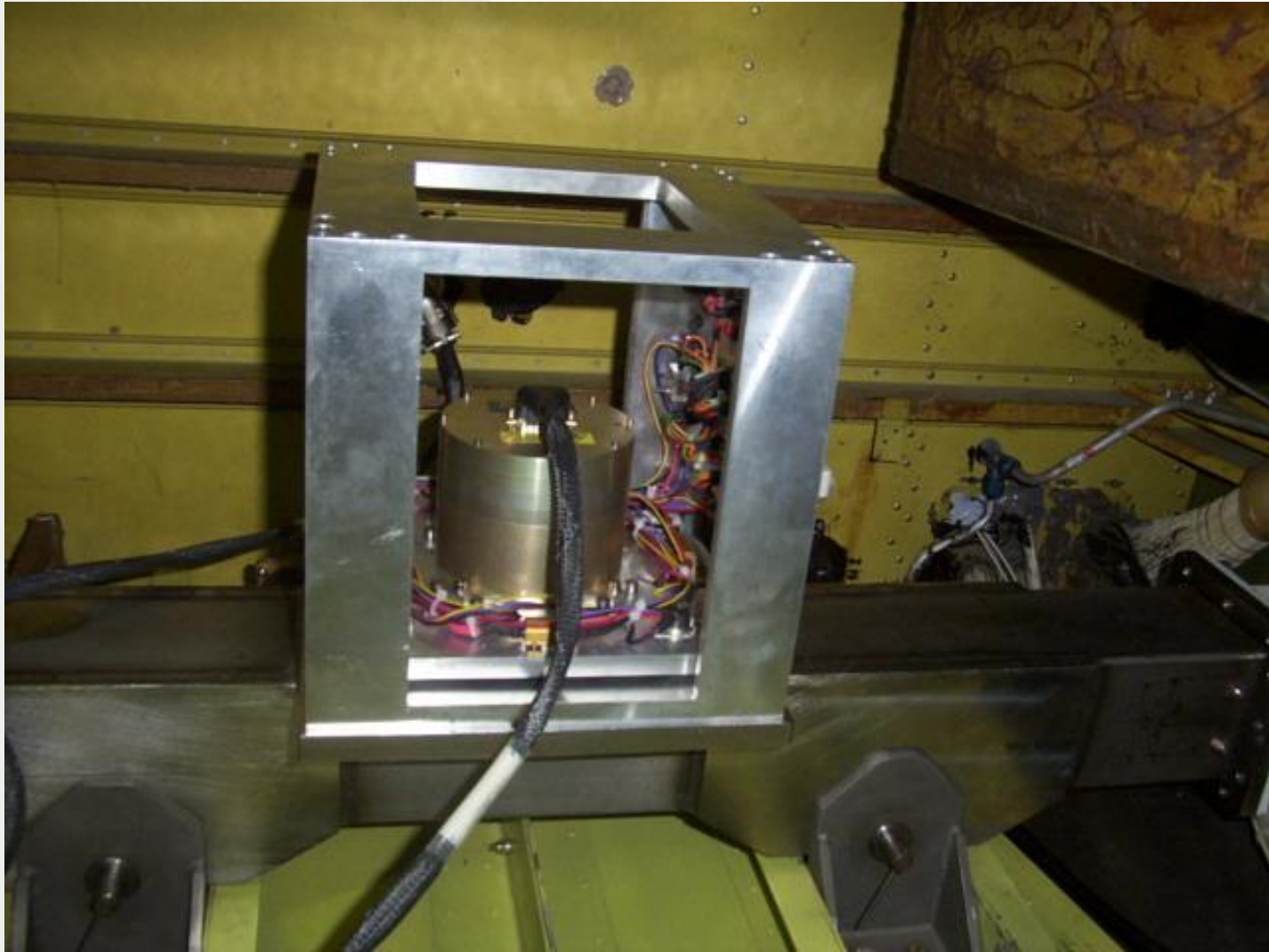
IMU mounted on the beam
