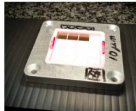
Alignment of sensors in custom frame
