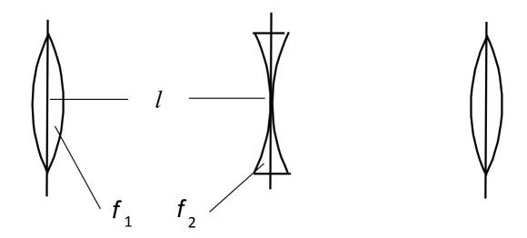
(b) A FODO cell (from mid-F, through D and to the midpoint of the next F) may be considered to be one such matrix with  $f_1 = +2f$  and  $f_2 = -2f$  followed (and multiplied) by another matrix with  $f_1 = -2f$  and  $f_2 = +2f$ . Using the result of the last question, write down these two matrices and show by taking their product that the matrix for a FODO cell from mid-F quadrupole
