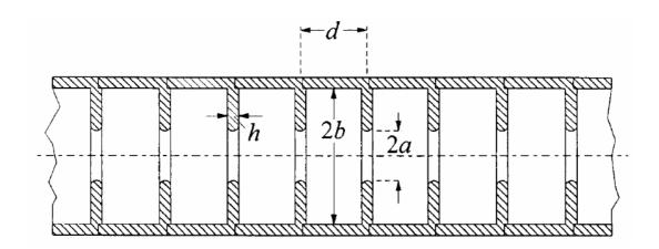
Assuming that the cavities are operated in the  $2\pi/3$  mode with a phase velocity  $\beta_z = 1$  and a supplied power of 35 MW, what is the total accelerating voltage and energy gain per metre for a SLAC structure of length l = 3 m.?
