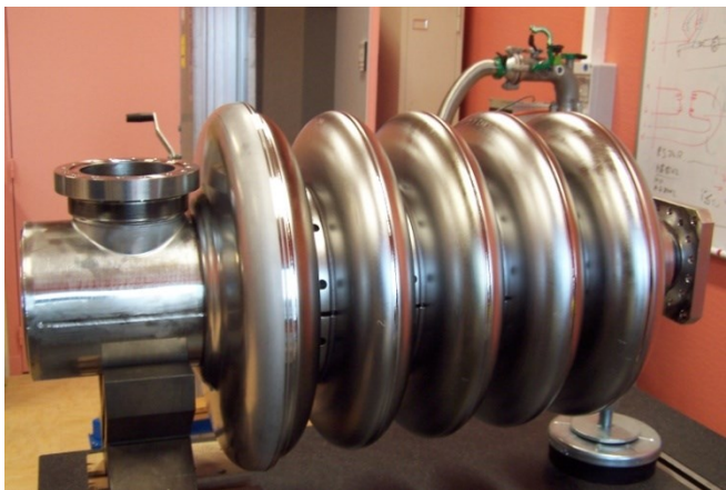
INFN & CEA 704 MHz elliptical SC cavities
