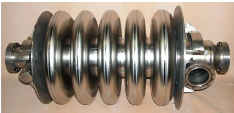
INFN & CEA 704 MHz elliptical SC cavities
