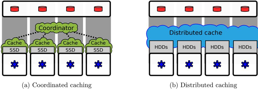
Figure 2: Caching Scenarios: Coordinated caching uses isolated caches, which form a single service via coordination. Distributed caching forms a single cache, which is delocalised across multiple hosts.
