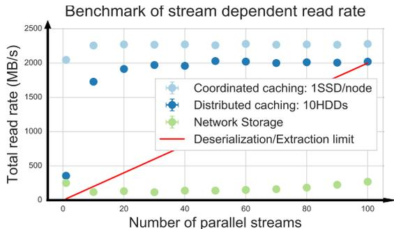
Figure 3: Performance of data sources: Throughput of synthetic, concurrent data streaming. All streams are equally distributed across 4 processing hosts. SSD and HDD devices are local to hosts, while network storage is shared. The Deserialisation/Extraction limit is extrapolated from analysis workflows.
