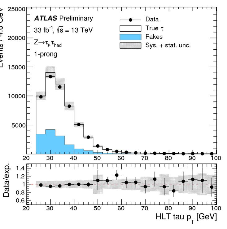
FAR LEFT: Tau probes passing requirements including a 25 GeV minimum p<sub>T</sub> cut at the HLT reveal a plateau efficiency of 95% for 1-prong (shown) and 85% for 3-prong events.
