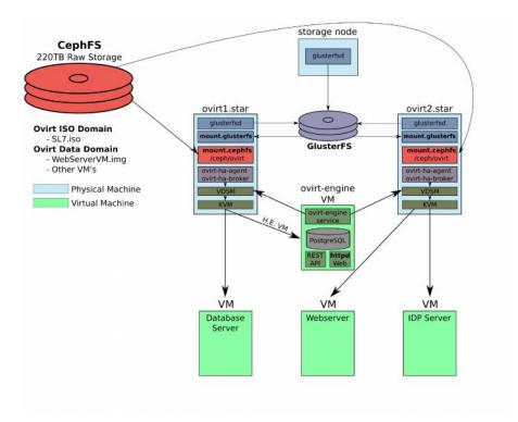
**Figure 2.** The diagram above is showing a Self-Hosted Engine oVirt Deployment where the oVirt engine is a highly available virtual machine itself. The GlusterFS filesystem is shown setup on ovirt1.star, ovirt2.star and a 3<sup>rd</sup> host titled storage node. The oVirt engine VM is stored in GlusterFS, the remaining VM's are all stored in CephFS.
