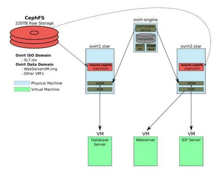
**Figure 1.** The diagram above is showing a Standard oVirt Deployment that is widely used within the oVirt community. The oVirt-engine is shown as the master node and the ovirt-engine service is shown managing the Virtual Desktop and Server Manager (VDSM) on the hypervisor nodes. CephFS is the main storage domain which is required to be mounted on all hypervisor nodes.
