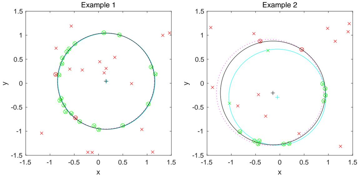
**Figure 1.** Two examples of fitted circles. Cyan: true circle with true center, green: signal points, red: background points, circled: points tagged as inliers by the M-estimator, magenta dotted: LMS circle, black: final circle with final center
