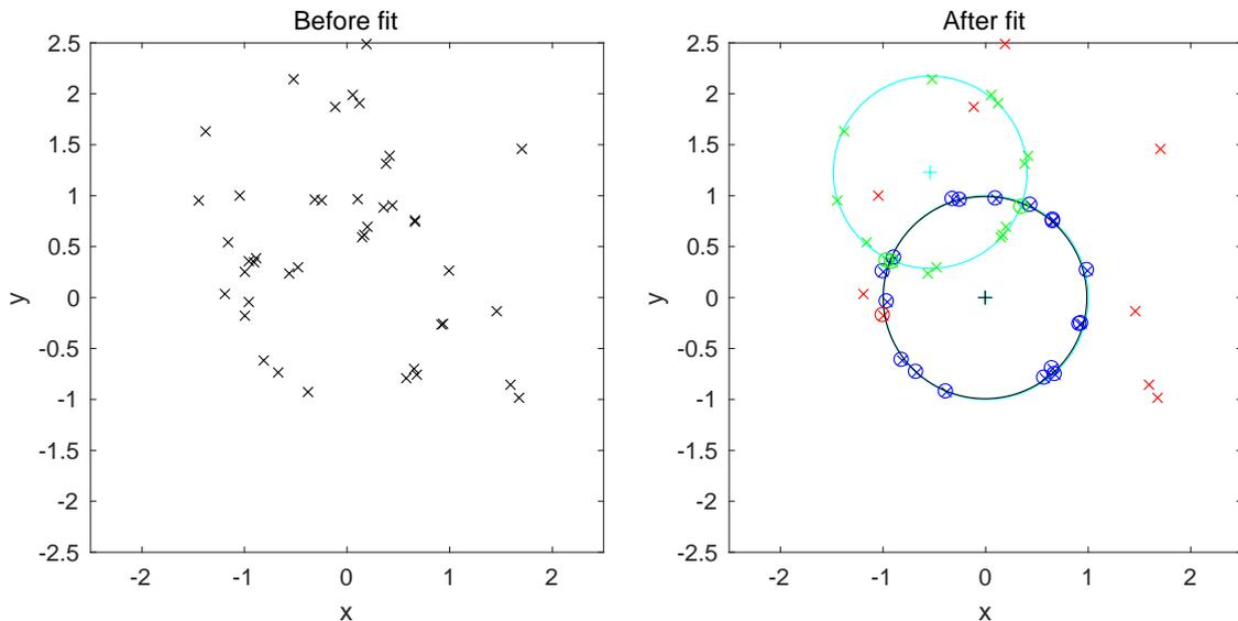
**Figure 2.** An example of a successful fit with overlapping circles. Left: all points before the fit. Right: after the fit; cyan: true circles with true centers, blue: signal points of the primary circle, green: signal points of the secondary circle, red: background points, circled: points tagged as inliers by the M-estimator, black: final circle with final center
