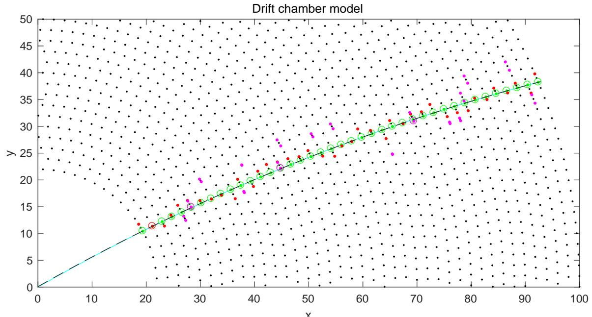
**Figure 3.** An example of a track at noise level  $p_N = 0.4$ . Cyan: true track, green: true points, red: mirror points, magenta: noise points, circled: points included in the track, black: final track.
