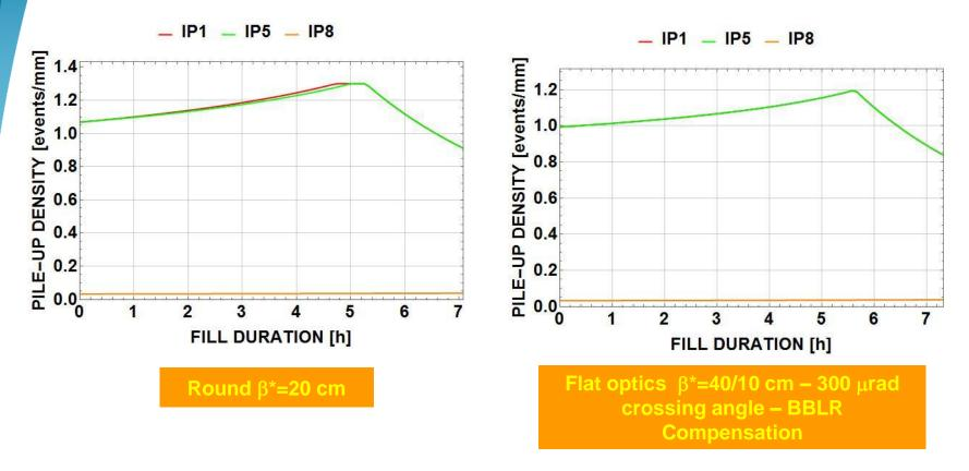
Marginal gain wrt integrated performance (+2%) but visible reduction of the pile-up density
