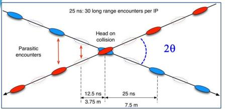
β\* levelling allows operating with larger long range beam-beam separation when the bunch population is larger
