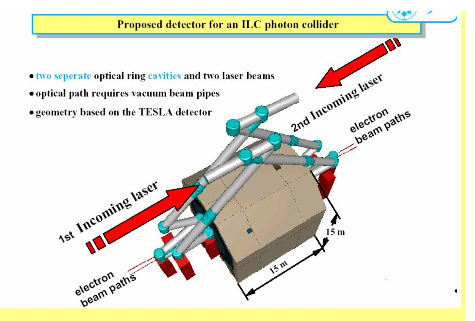
Design study of an optical cavity for a future photon-collider at ILC " G. Klemz , K. Moenig , I. Will
