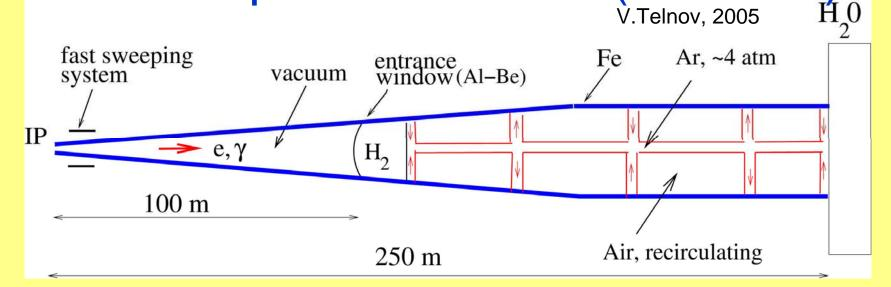
The photon beam produces a shower in the long gas (Ar) target and its density at the beam dump becomes acceptable.
