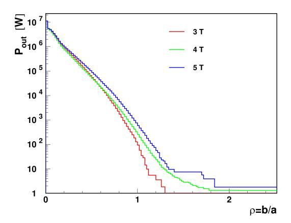
Increasing the vertical opening by 50% we decrease the power dissipation by  $\sim$  2 orders of magnitude
