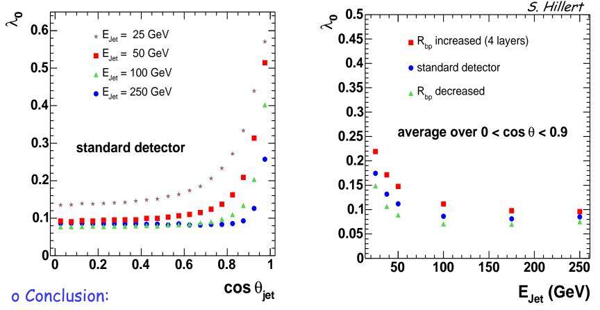
vertex charge performance strongly depends on low momentum tracks  $\rightarrow$  differences between designs most pronounced for low jet energy and large cos  $\theta_{jet}$
