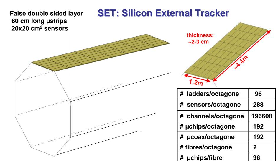
Total surface: ~86 m<sup>2</sup> Nb channels: 1,572864 Nb of fibres: 8 per side
