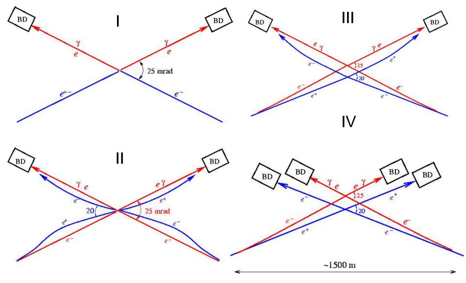
The scheme 1 is the simplest and cheapest. All the same for e+e- and  $\gamma\gamma$  (only smaller  $\beta_x$  for  $\gamma\gamma$ ). Why not? Because in e+e-there is a special extraction line for measurements of energy and polarization of final particles. Is it really needed? This
