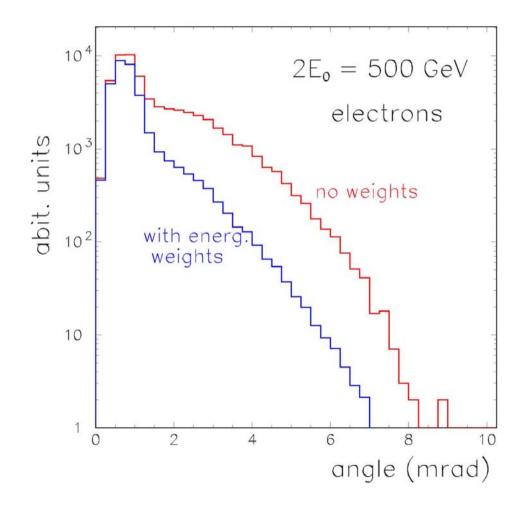
If the beam dump is situated at L=250 m, than for particles with  $\theta$ =7 mrad r~1.8 m, too much. Some focusing of electrons will be useful in order to decrease the radius of the tube and to reduce the energy deposition (rad. activation on the way to the beam dump).
