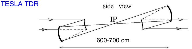
Then the diameter of focusing mirror is about 20 cm and that of the auxiliary mirror about 11 cm. The dead angle for tracking remains as before about ±95 mrad, for calorimetry smaller. The laser density is far from the damage threshold, the average power is the most serious problem.
