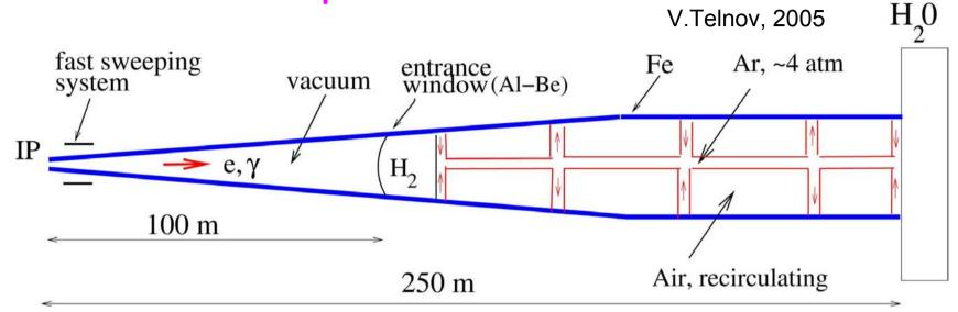
The photon beam produces a shower in the long gas (Ar) target and its density at the beam dump becomes acceptable.
