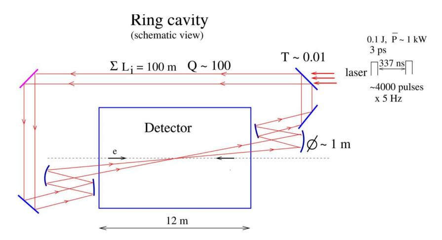
The cavity includes adaptive mirrors and diagnostics. The required tolerances are small, but in gravitation detectors they are 10<sup>9</sup> times smaller.
