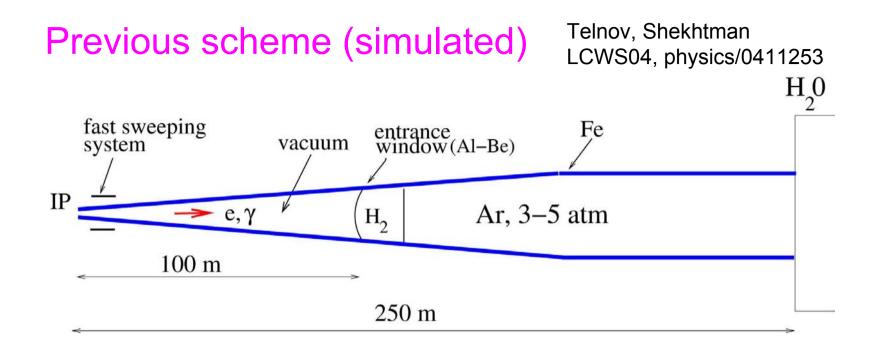
Max.  $\Delta T$  in water after one train at 250 GeV photons is 75,50,25 at Ar pressure 3,4,5 atm.  $\Delta T$  at entrance window is about 40° C.
