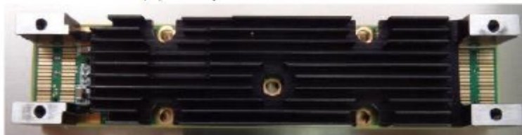
(c) A FECi with its heat sink
