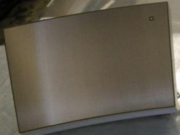
Resistive Kapton ~4 M \Omega / \square
