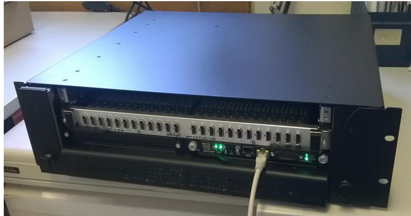
Photo SRS Minicrate with 1 blade, 24 HDMI ports for 6 kchannels
