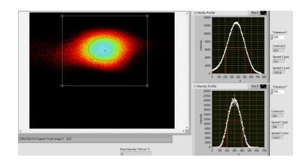
CAM5: Virtual exit of vapor source FWHM: X: 2.8 mm Y: 2.3 mm Peak Intensity: 10 TW/cm^2 1mm X: 7 TW/cm^2 1mm Y: 6 TW/cm^2
