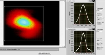
CAM4: Virtual center of vapor source FWHM: X: 1.6mm Y: 1.1mm Peak Intensity: 40 TW/cm^2 1mm X: 10 TW/cm^2 1mm Y: 4 TW/cm^2
