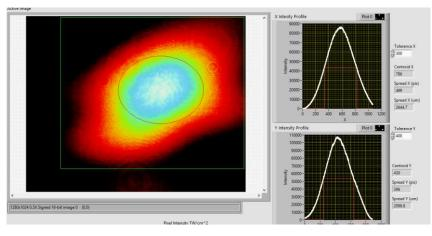
CAM3: Virtual entrance of vapor source FWHM: X: 2.1 mm Y: 1.2 mm Peak Intensity: 20 TW/cm^2 1mm X: 3 TW/cm^2 1mm Y: 15 TW/cm^2
