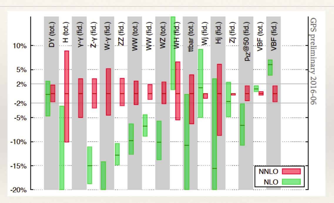
\* This plot (by Salam) indicates that NNLO (central value) lies within the NLO error band (based on scale variation) in only 3 cases out of 17.
