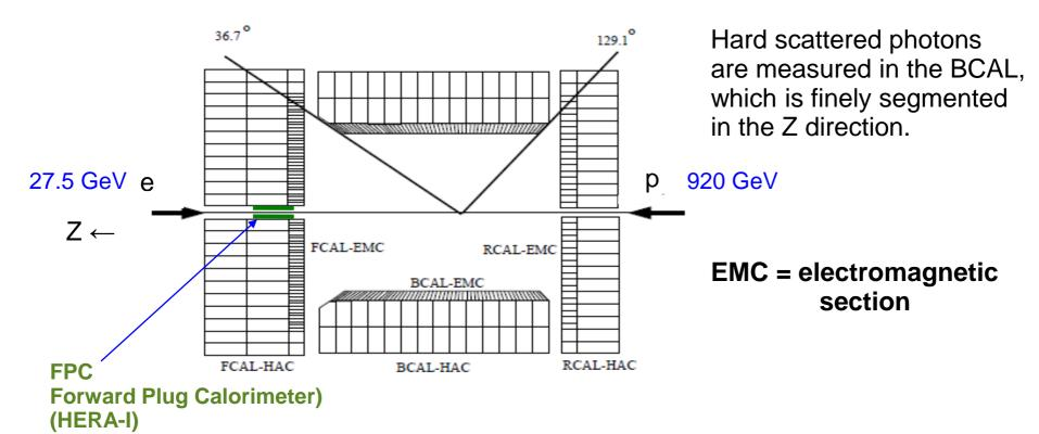
Replaced by a beam focussing Magnet In HERA-II
