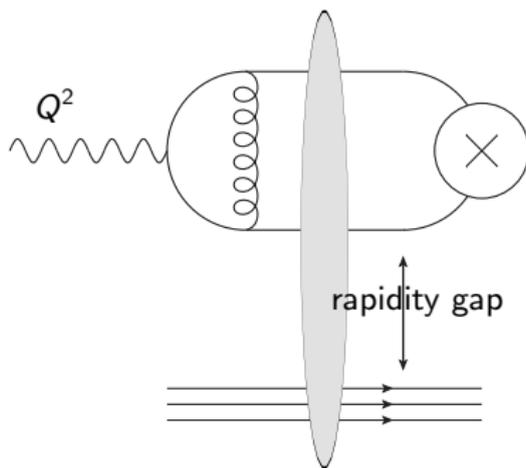
Amplitude for diffractive  $V$  production
